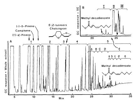
Fig. 1. Gas chromatograms (FID) of volatiles from a 40-male-infested Norway spruce log ( $25 \times 8$  cm diam.). Numbers and letters above peaks indicate the effluent collection periods for the respective fractions. Methyl (E,Z)-2,4-decadienoate cannot be discriminated visually in chromatogram A on a polar GC phase (column 1, Table 1) but was located by EICP-GC-MS and can be seen in chromatogram B as a small side peak (non-polar GC phase, column 3).
